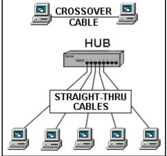
The next step up would be a network consisting of three or more computers and a hub. Each of the computers is plugged into the hub with a straight-thru cable (the crossover function is performed by the hub).
