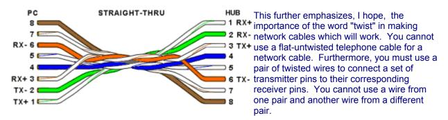
Keeping the above principles in mind, we can simplify the diagram for a 568A straight-thru cable by untwisting the wires, except the 180° twist in the entire cable, and bending the ends upward. Likewise, if we exchange the green and orange pairs in the 568A diagram we will get a simplified diagram for a 568B straight-thru cable. If we cross the green and orange pairs in the 568A diagram we will arrive at a simplified diagram for a crossover cable. All three are shown below.
