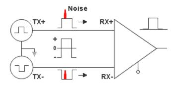
Pulses of energy travel down the transmission line at about the speed of light (186,000 miles/second). The principal components of one of these pulses of energy is the voltage potential between wires and current flowing near the surface of the wires. This energy can also be considered as residing in the magnetic field which surrounds the wires and the electric field between the wires. In other words, an electromagnetic wave which is guided by, and travels down the wires.
